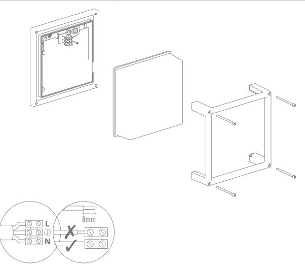
Note: -The lamp must be installed by professional electrician -Ensure the power supply is switched off before fitting this product -Do not touch the lamp when in use -Keep away from hot steam and corrosive gas
